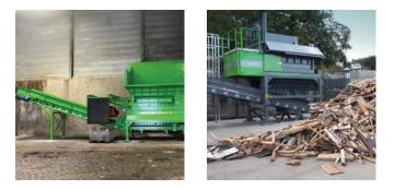
RENTEC build screens for the correct separation of fines (ECODISC®) or for the removal of oversized parts (SCALPEL) to avoid clogging in the subsequent separation line. Together with MECBIO, they build turnkey shredding and screening solutions completed with a total range of modular conveyor systems.
