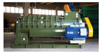
The Ecomade Separators are made for processing Biowaste or de-packaging food waste. Built with a sturdy steel frame equipped with inspection doors. Inside, a rotor equipped with special hammers and mallets makes a division of the material to separate
